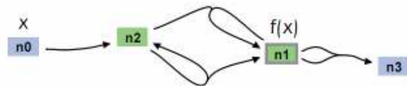
Fig.1: A network where the concentration of n1 is the cube-root of the concentration of n0
